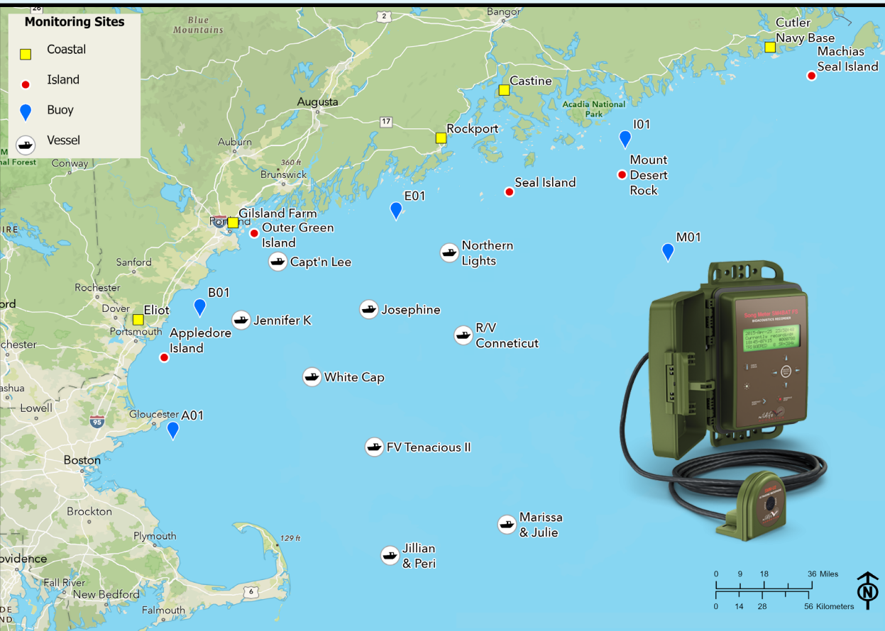
Figure 1. Above: Map of monitoring sites in the Gulf of Maine. Overlay: Wildlife Acoustics SM4 bat detector used to listen for bat calls.
