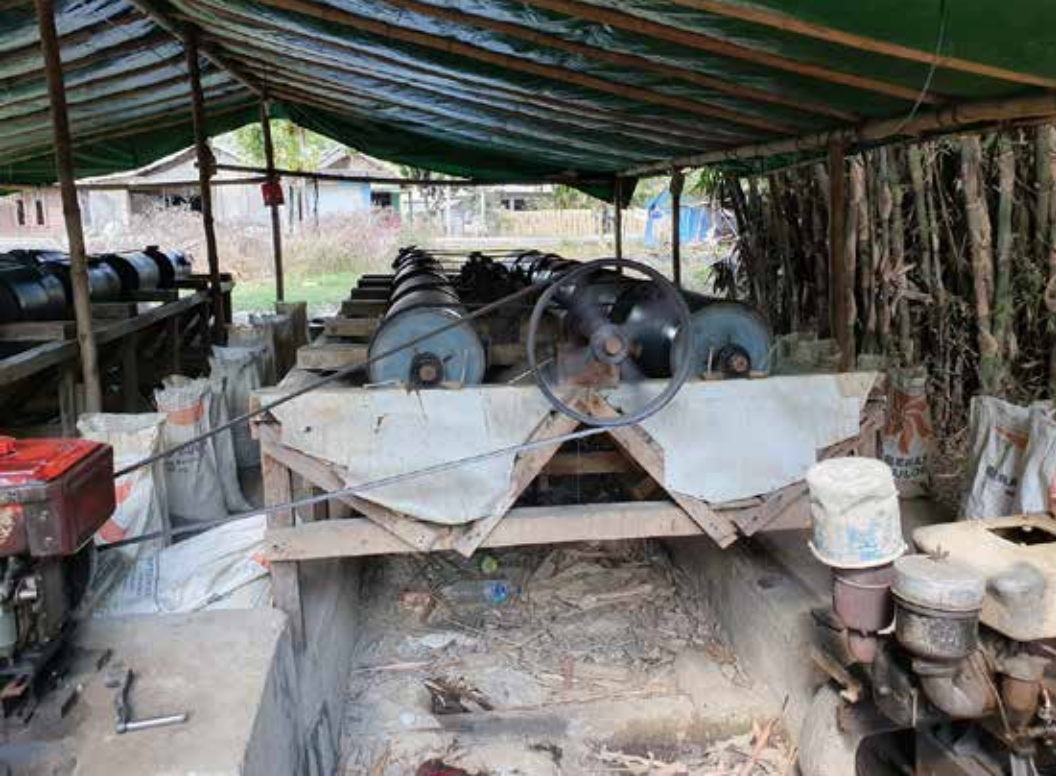
Figure 1. Example of an Indonesian ball mill 'processing centre' for gold ore.
