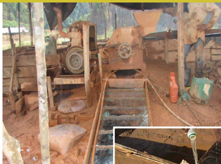
The use of copper plates for whole ore amalgamation in the Tapajós River Basin. Photo: Global Mercury Project
