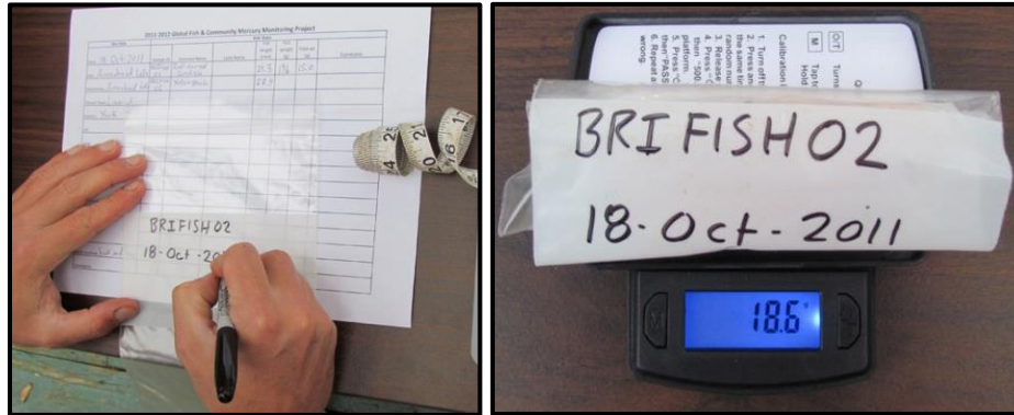
Figure 5. It is important to record the sample ID clearly and accurately. Place the cleaned fillet into the labeled bag. Remove all air from the bag and fold. Place the fillet sample on the tared, pocket-size scale. Record the fillet weight on the sample data sheet.
