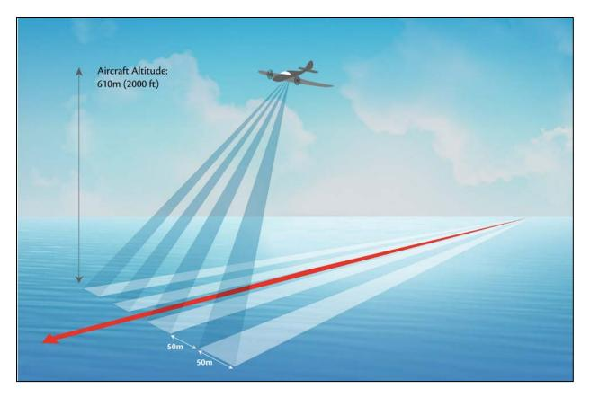
**Figure 3-2.** Digital video aerial surveys were flown at 610 m using a twin-engine aircraft with four belly mounted cameras. These cameras recorded non-overlapping 50 m transect strips, for a 200 m total transect strip width.
