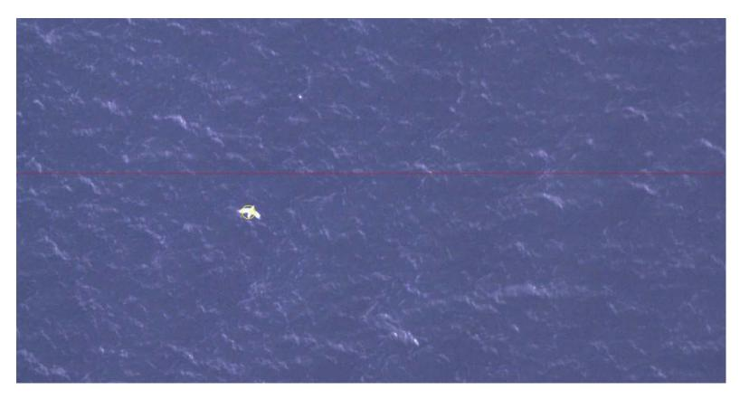
Figure 4C-2. Gain can be adjusted to help pick up different features on the object for identification. Here, gain was increased from the base image in Figure 4C-1, causing the white on this bird to stand out.
