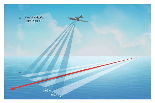
**Figure 3-3. Digital video aerial surveys were flown at 610 meters using a twin-engine aircraft with four belly mounted cameras.** These cameras recorded non-overlapping 50 meter transect strips for a total transect strip width of 200 meters. (Image created by Linda Mirabile and Glen Halliday).
