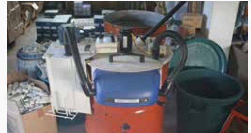
Bulb crushers are installed at recycling centers in some countries. Next steps include waste management and disposal.
