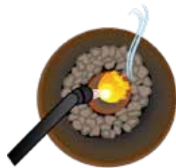
Mercury/gold amalgam heated to evaporate Hg
