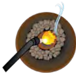
Mercury/gold amalgam heated to evaporate Hg
