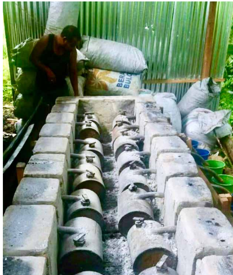
Cinnabar, the most common source ore for refining elemental mercury, is associated with recent volcanic activity. Cinnabar mines are used for supplying mercury in the country for ASGM activities. Above: A smelter to refine cinnabar for useable mercury.
