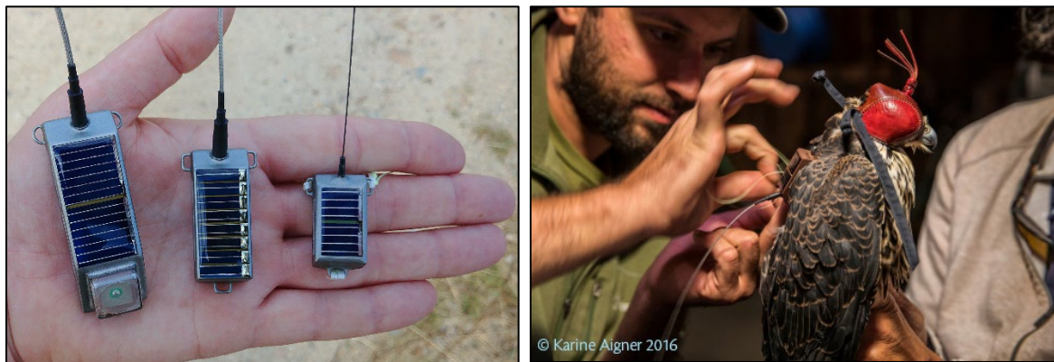
Figure 8. Left: Example of 22g solar GPS PTT unit, 12g solar PTT and 5g solar PTT unit used to track movements of Peregrine Falcons, Merlins and Northern Harriers. Right: A hooded Peregrine Falcon being fitted with a transmitter (right).
