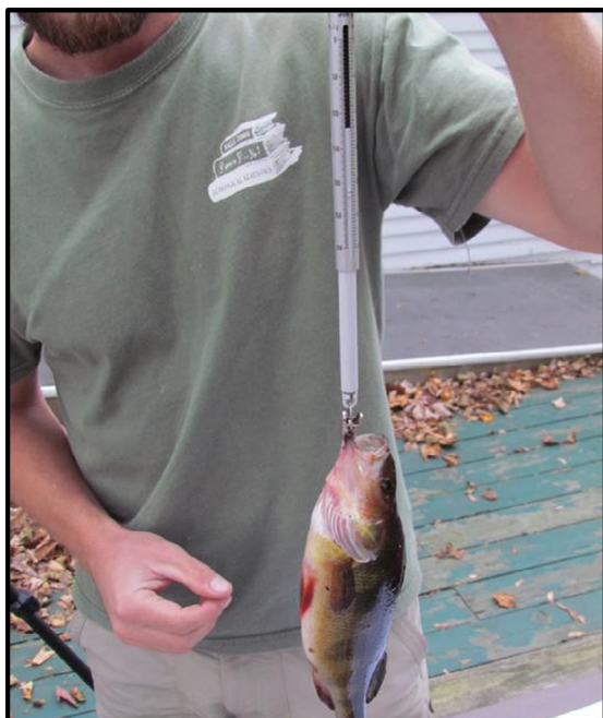
Figure 2 (left) and 3 (right). Taking the total weight (to the nearest 0.1 g) and total length (to the nearest 0.1 cm) of a fish. These data are used to interpret the results of mercury analysis and allows for comparisons across multiple sampling sites.
