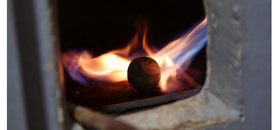
Burning amalgam to vaporize mercury is commonly used in artisanal and small-scale gold mining and releases toxic mercury vapor into the atmosphere.
