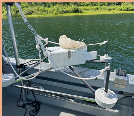
Our staff developed a sediment trap to capture potentially contaminated suspended sediments entering tribal waters in the Upper Columbia River.
